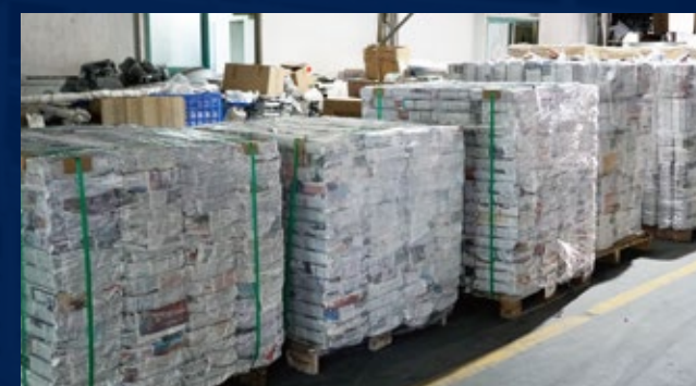
Single wrapped newspaper + electrostatic film + wooden support
